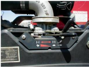
Start the engine at an idle then slowly bring the RPM's up, giving the cutting wheel time to build up speed.
