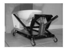
STEP 1 Close water supply valve. Remove supply line. Roll jack under toilet bowl. Raise the lifting arms to support the weight of toilet.
