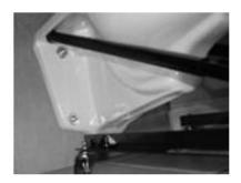
STEP 2 Remove both left and right side nuts and washers.
