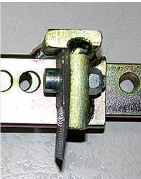
WARNING Improper use of this tool will bend the teeth straight. This item is not covered by the Equipment Protection Plan. Note: this picture shows the proper curve of a tooth.
