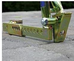
The tool will touch the top of the pavers on both ends when properly inserted. (as shown)
